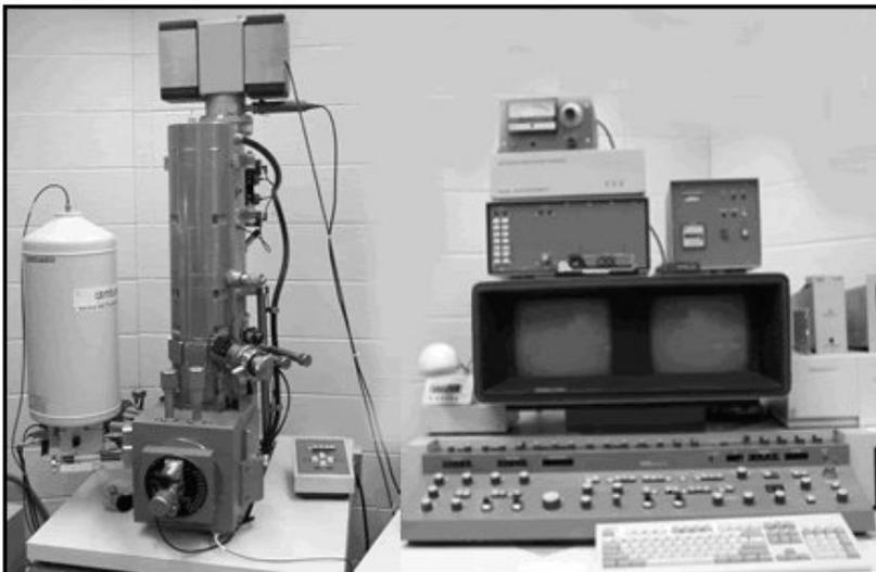
The Geoscience Department's electron microscope and energy dispersive x-ray spectrometer.
