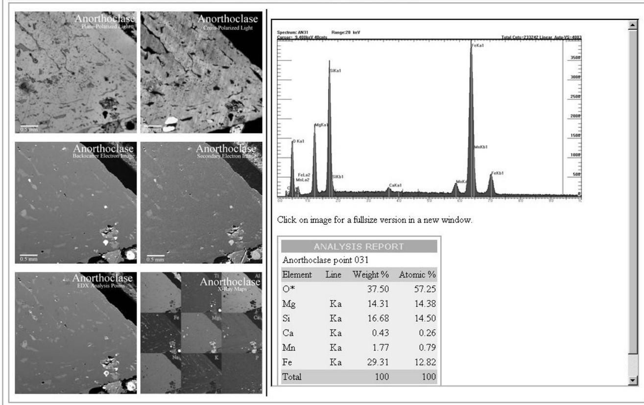
**Figure 3. Choosing a point (here point 31) places the EDX spectrum and an analysis report in the right-hand window. This image can be expanded for easier examination.**
